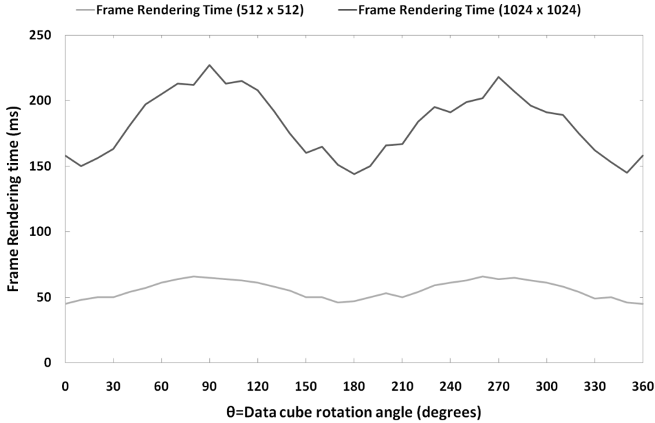
Figure 12: Single frame rendering times for different cube rotation angles with different output sizes ( 1024 \times 1024 and 512 \times 512 pixels). The timing measurement was done for the HIPASS cube on 3 workstations (one acting as a server) and 4 GPUs (2 P 4 G).
